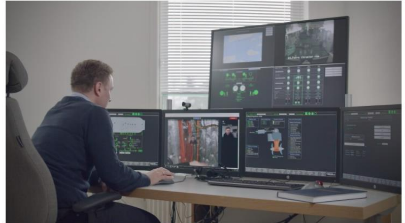
Kim Gunnar Jensen, project engineer at Fjord1, at the shore-based engine control centre used in the ROMAS project. PHOTO: Fjord1
