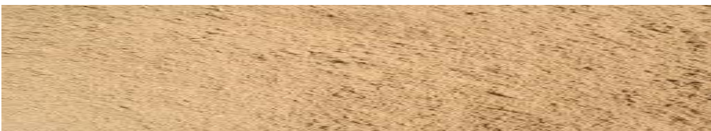
Sand: Shell sand / building sand – Abrasion test Miller No. 30 (< 50 = non-abrasive)
