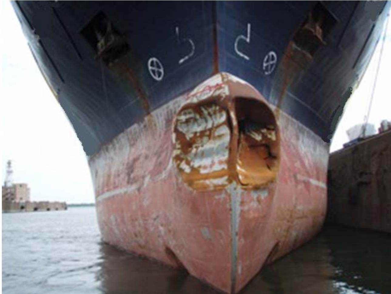
Damage to bulbous bow in 2008
