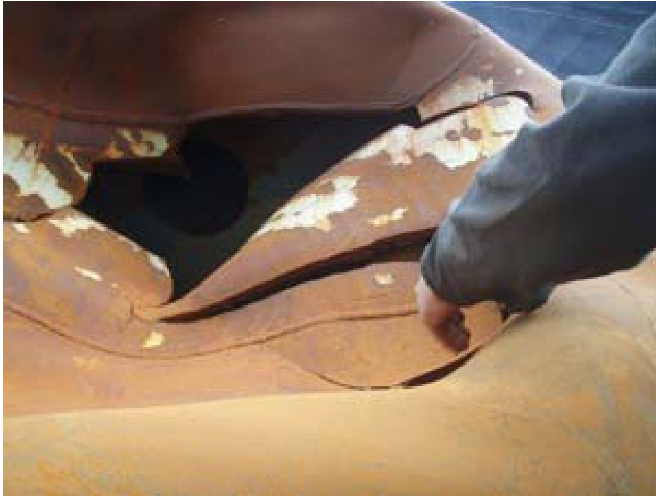
Puncture through bulbous bow.
